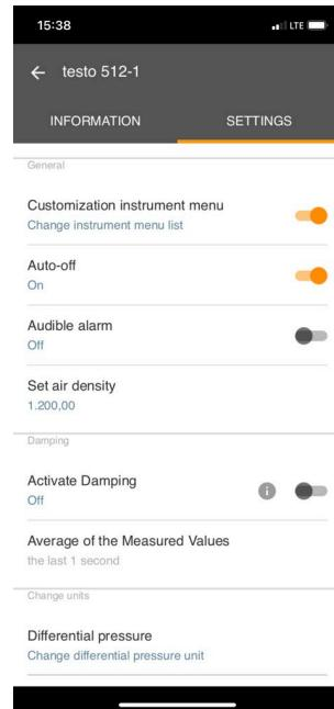
Changes to the measuring instrument settings in the app are transferred directly to the measuring instrument. Synchronization with the app is confirmed on the measuring instrument via "SYNC DONE".
